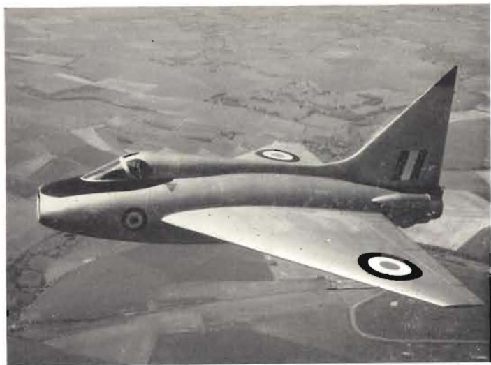
THE BOULTON PAUL P.111. This tailless, delta-wing aircraft has been designed for high-speed aerodynamic research, and is powered by a Rolls-Royce Nene turbojet engine. Its span is 33 ft. 6 in., length 26 ft. 1 in., height over fin 12 ft. 6½ in. All other details are secret.
