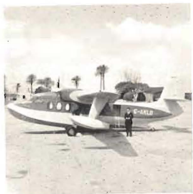
THE SHORT SEALAND. A 5 to 8-seater amphibian powered by two Gipsy Queen 70 engines, each of 345 b.h.p. Span 59 ft., length 42 ft. 2 in., maximum speed 164 knots, cruising speed 152 knots.
