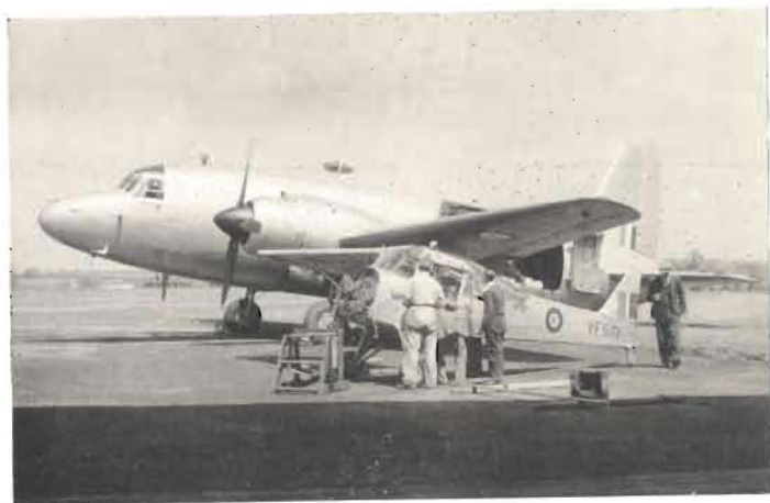
THE VICKERS VALETTA. An R.A.F. transport version powered by two Bristol Hercules 230 engines of 1,975 h.p. each. Wing span 89 ft. 3 in., length 65 ft. 2 in. An Auster Mk. 6 is seen here being dismantled for transport from Wymeswold to Singapore in the Valetta.
