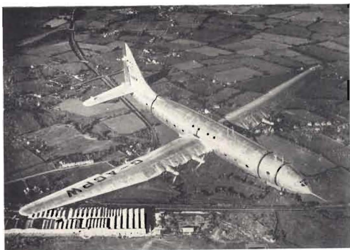
THE "BRISTOL" BRABAZON I, MARK I, powered by eight "Bristol" Centaurus sleeve-valve engines driving four pairs of co-axial, contra-rotating airscrews; it has a wing span of 230 ft. and a length of 177 ft.
