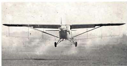
The Auster Aiglet equipped for crop spraying. (One gallon per acre installation)
