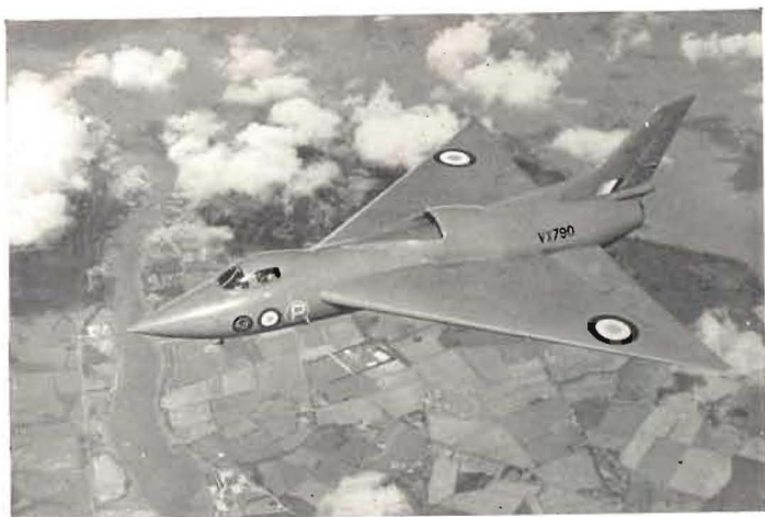
THE AVRO 707B. A single-engined delta-wing research aircraft powered by a Rolls-Royce Derwent. This aircraft was built primarily in order to examine wind-tunnel theories on the delta-wing configuration.
