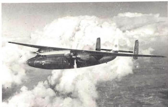
THE AIRSPEED AMBASSADOR, a 40/47-seater medium-stage airliner powered by two Bristol Centaurus engines of 2,600 b.h.p. each. The economical cruising speed is 240-260 m.p.h., and a stage-length of 1,000 miles can be flown while carrying 36 passengers and their luggage.
